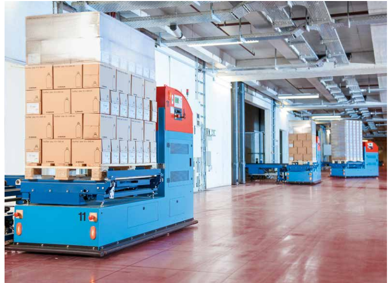
6 WLAN-controlled transport vehicles take the pallets to the high-bay storage area. En route, the boxes are gamma sterilized.
