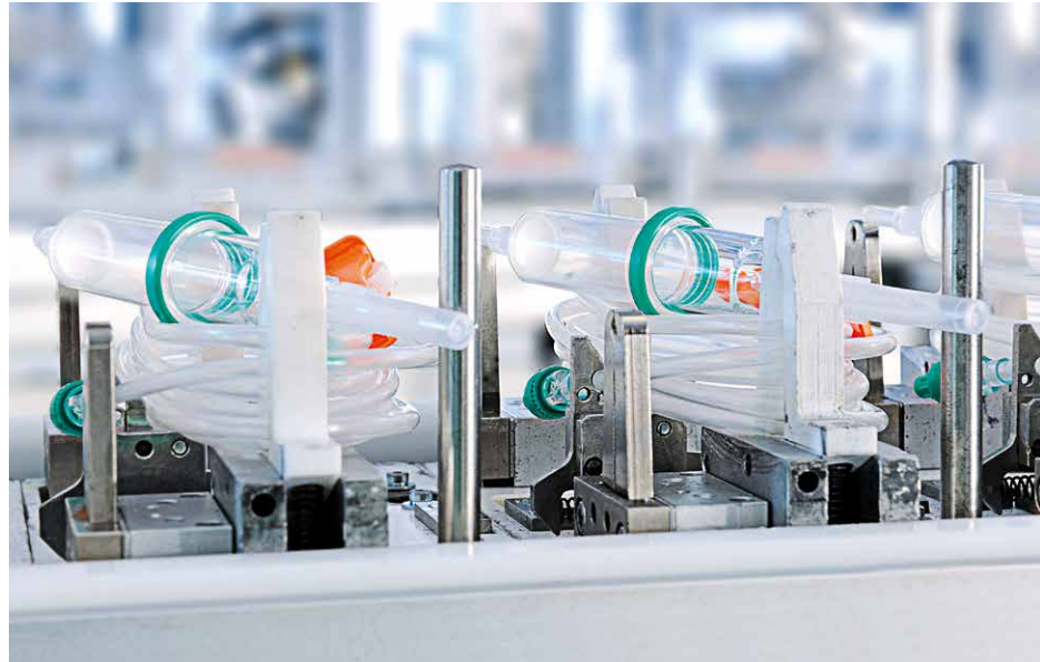
4c The individual parts of the Intrafix® SafeSet are transported to the final assembly area on conveyor belts. They are glued and welded together under continuous quality control.
